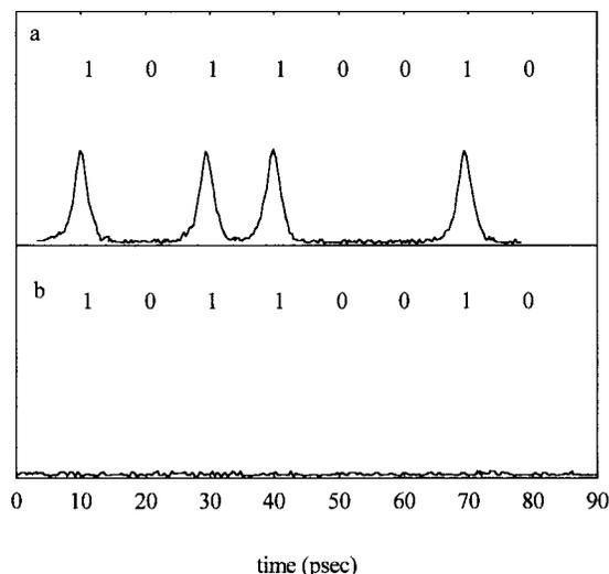
Fig. 4. Cross-correlation results of the output of the packet router. (a) The incoming header does not match the local header (packet sent back to network); (b) The header matches the local header (packet sent to demultiplexer).
