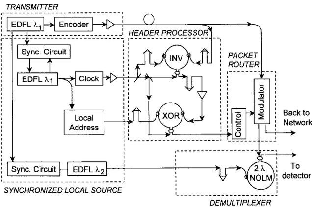
Fig. 1. Detailed diagram for the packet-drop experiment. The transmitter consists of a master laser and a packet encoder. The packet-drop part consists of synchronized local lasers, a local header generator, a clock pulse train generator, a header processor, a packet router, and a demultiplexer. INV—inverter, XOR—exclusive OR gate, 2- $\lambda$  NOLM—two-wavelength nonlinear optical loop mirror, and EDFL—erbium-doped fiber laser.
