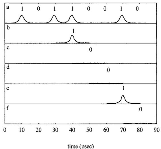
Fig. 3. Autocorrelation results of the demultiplexer. (a) Input data packet; (b)–(f) Output of the 2- $\lambda$  NOLM by adjusting the delay of the local pulse by an additional 10 ps each time.
