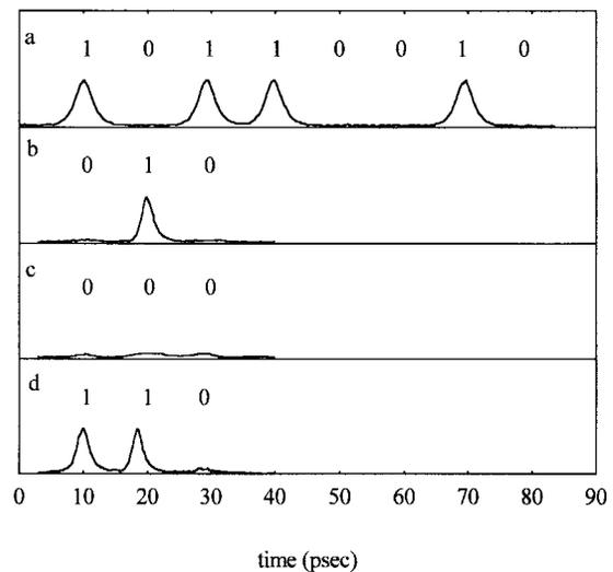
Fig. 2. Cross-correlation results of the header processor. (a) Input data packet; (b) Output of the inverter; (c) Output at the XOR gate when the headers match; and (d) Output at the XOR gate when the headers do not match (the inverted incoming header is 010 and the local header is 100).
